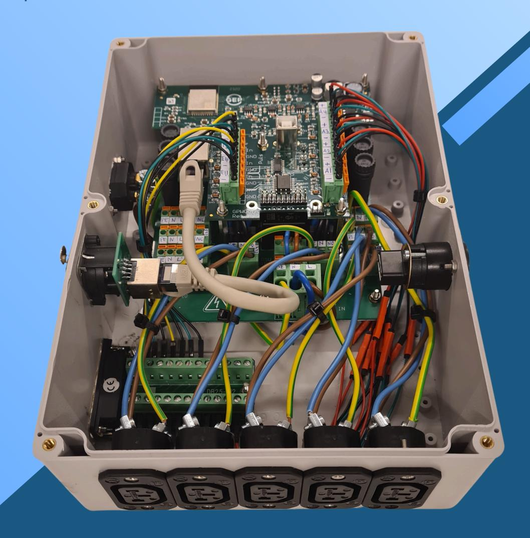
Lower Board: 8 relays | Output Upper Board: CPU | Input/Output
